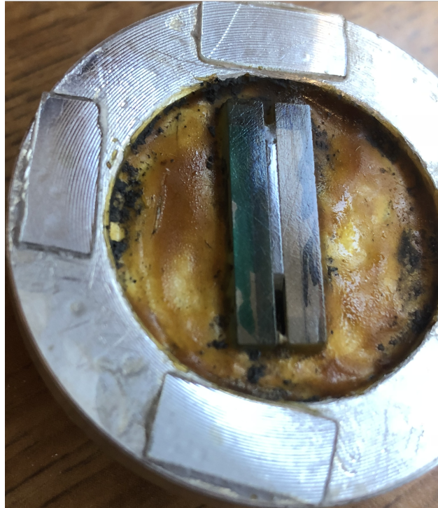
Figure 4. %8YSZ specimen laterally mounted with the help of gypsum. The thin layer in the center is the sectioned sample; the two wider layers at its sides are stabilizing glass; and the yellowish area is gypsum covered with resin. The resin prevents, during the polishing process, residual gypsum to fall on the polishing pads.
