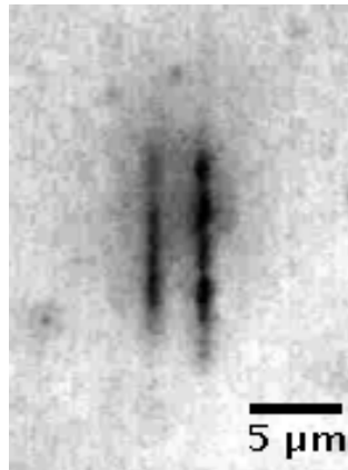
Figure 28. Optical micrograph in transmission of damage tracks across the nc-YSZ ceramic.
